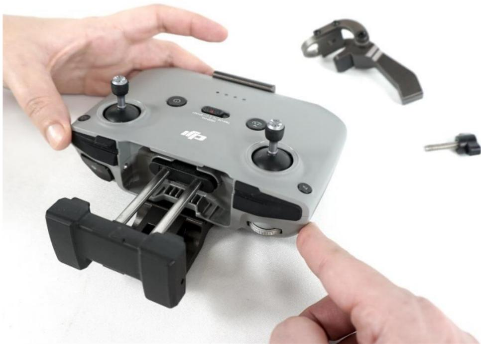
Reconnect the neck of the aluminum base between the antenna bars back to the main body.
