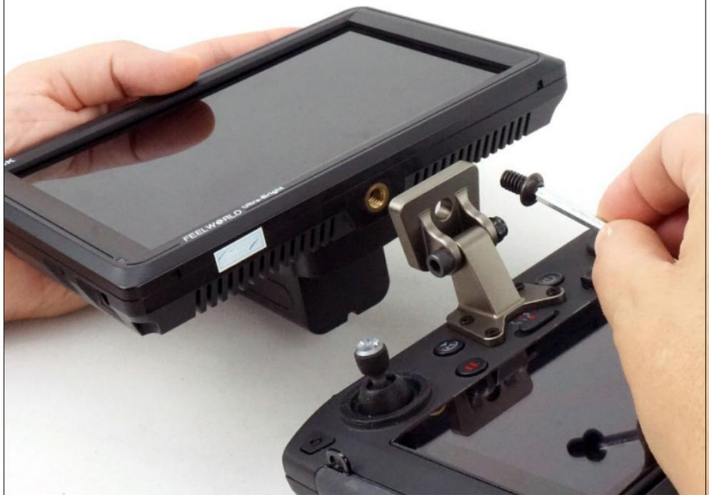
Adjust the position of the monitor, accordingly , use the hex key to tighten it in place. You can use a small wrench tool #8 (not provided) to give it an extra tight.
